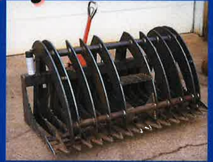
COMPLETED GRAPPLE BEFORE PAINTING
